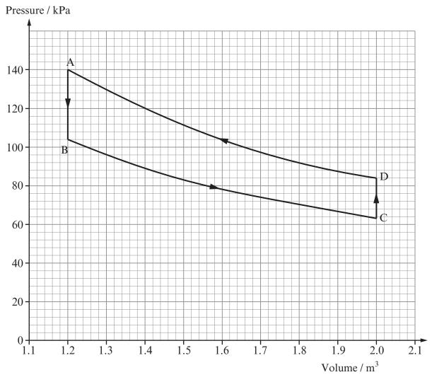
**BC** and **DA** are isotherms (the temperature along each of BC and DA is constant) and there are **49.3 mol** of ideal gas.
